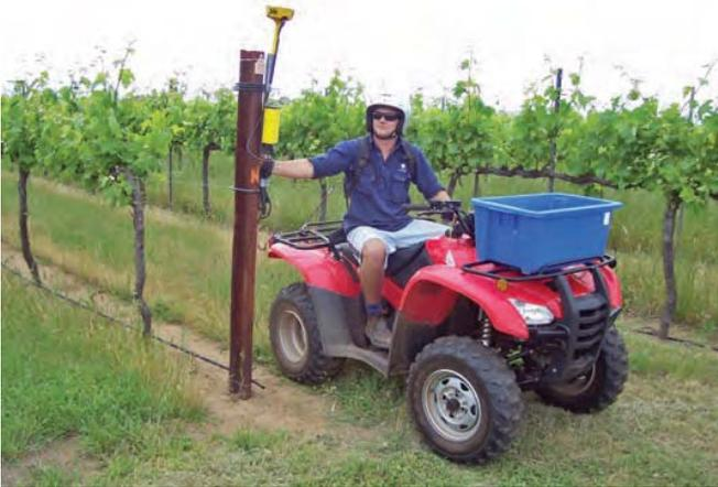
Fig. 1. Surveying block boundaries using a differential Global Positioning System (DGPS). Courtesy of Adams Road Vineyard, Margaret River, WA.
